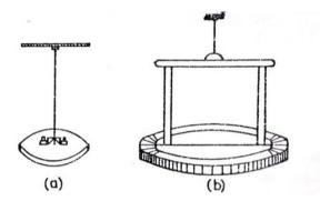
The torsion pendulum is formed by the given circular disc suspended whose rigidity modulus is to be determined. The experiment consists of three parts:
