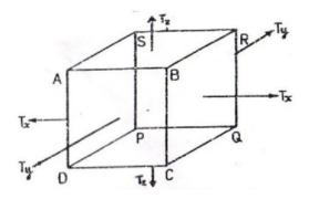
Fig 1.5 Application of bulk stress on a cube.
