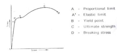
Fig 1.1 The Stress – strain curve for low carbon steelwire
