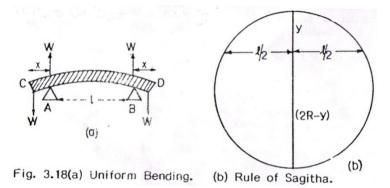
Consider a light beam CD supported symmetrically on two knife edges at A and B and loaded with equal weights W at each end as shown in the above figure. Hence the reaction at each knife edge is equal to W. Now the beam bends uniformly and forms an arc of a circle of radius R.
