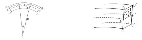
Let a beam ABCD having rectangular cross section be bent in the form of an arc of a circle of radius R with the centre at O. Consider a small portion ab of neutral axis of the beam subtending an angle  $\theta$  at the centre O. a'b' is another small portion of a filament at a distance 'z' above the neutral filament ab. Before bending a'b' = ab. After bending, a'b' > ab since a'b' is above the neutral surface.
